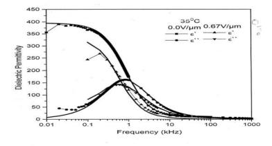
Fig. 1(a) Dielectric spectra as a function of frequency at 35°C without bias and at  $E = 0.67 \text{ V}/\Box \text{m}$  bias.
